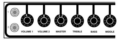
TREBLE: This control varies the amount of treble frequency in the preamp. The first in the series of tone controls, it is the most powerful of the three because its setting determines the amount of signal fed to the BASS and MIDDLE Controls. High settings of the TREBLE Control will greatly diminish the effectiveness of the BASS and MIDDLE, causing them to have very little effect on the sound.
